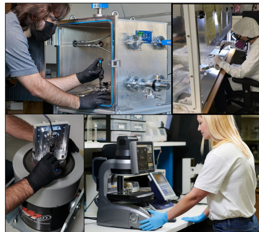
Figure 6. Thermal-vacuum chamber, laminar flow bench, precision measurement, vibration testing
